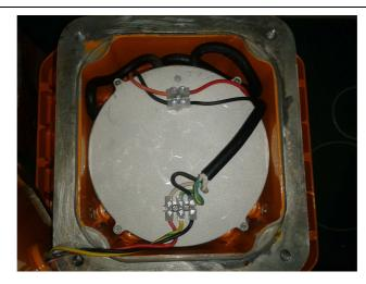
(This photo is close to the real product, pls reference it mainly when wiring. In the photo, the white and red wires are live lines, the black wires are neutral lines and the green/yellow is ground line) Connect each line rightly with the input terminal of the cable from the AC power source respectively by using screwdriver.
